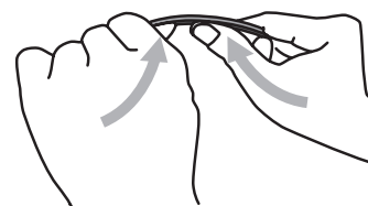
Along the wide flat side the craft stick is easy to break.
